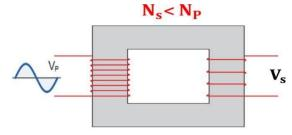
For a step down transformer the number of turns in the secondary will be less than that in the primary ( $N_s < N_P$ )
