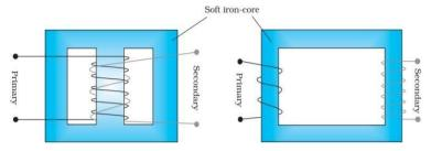
A transformer consists of two sets of coils, insulated from each other. They are wound on a soft-iron core, One of the coils called the primary coil has  $N_P$ turns. The other coil is called the secondary coil; it has  $N_S$  turns. Often the primary coil is the input coil and the secondary coil is the output coil of the transformer.
