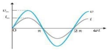
In a pure resistor, the voltage and current are in phase. The minima, zero and maxima occur at the same. Phasor diagram for the circuit
