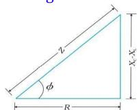
The phase difference  $\phi$  can be obtained using impedance diagram.
