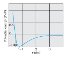
A rough plot of the potential energy between two nucleons as a function of distance. The potential energy is a minimum at a distance  $r_0$  of about 0.8 fm.
